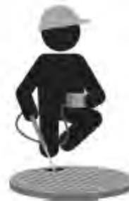
j) Determine safe oxygen and gas levels using a gas meter. If safe, insert air exchange / exhaust fan hose.
