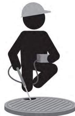
Measuring safe gas levels before opening tank cover.
