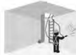
Cleaning man-entry tanks with pressure jet wash
